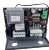
AS07300 (SR302 - 868 MHz) Control unit with on-board radio receiver See page 120
