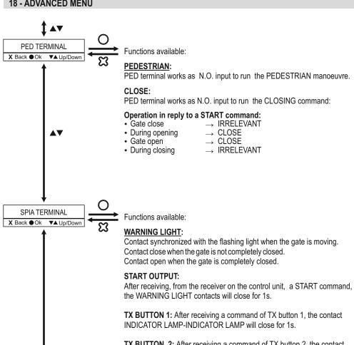
**TX BUTTON 2:** After receiving a command of TX button 2, the contact INDICATOR LAMP-INDICATOR LAMP will close for 1s.
