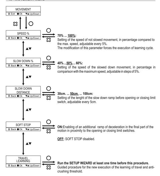
During the learning of travel and anti-crushing threshold, the intervention of safety devices or the activation of command inputs determines that the procedure has not been successful and it will be necessary to repeat it.
