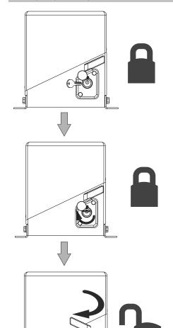
Rotate the unlocking device cover and put the key into the cylinder
